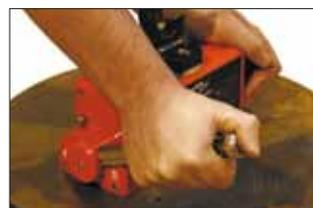
To Switch the lifter OFF return the load to the floor or support. Depress the plunger on the handle and rotate 120° clockwise to its stop position. Release the plunger to complete the switching process.
