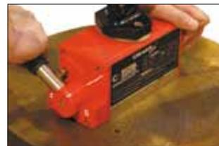
To Switch the lifter ON rotate the handle 120° anti-clockwise.
