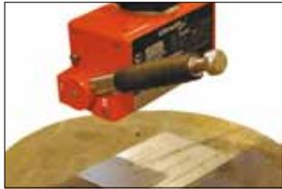
To pre-test any load, place the Safety Shim on the load and lower the Ultralift on to it.
