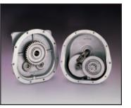
Precision spur machined from high-alloy steel or drop forgings and case hardened for long life and quiet operation. Gearing operates in a precision machined ductile iron or steel gearcase and is continuous oil bath lubricated to reduce maintenance and increase life.
